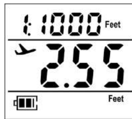
1.000 – 9.990 Altitude display: 10s Increments of 10 feet / 10 meters
