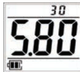
Temperature (Celsius) Battery voltage (V)
