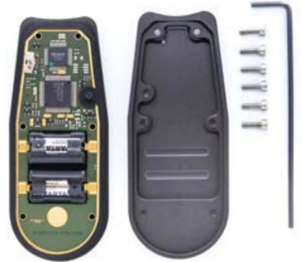
**WARNING:** The battery cover and seal must be installed correctly, using correct screws and torque
